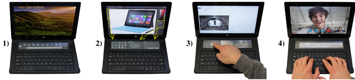
Figure 2. Example Application Scenarios: 1. Secondary Display Taskbar; 2. Dynamic UI Manipulation; 3. File Navigation and Manipulation; 4. Support for Concurrent Applications (e.g. Video call + Email Client)
