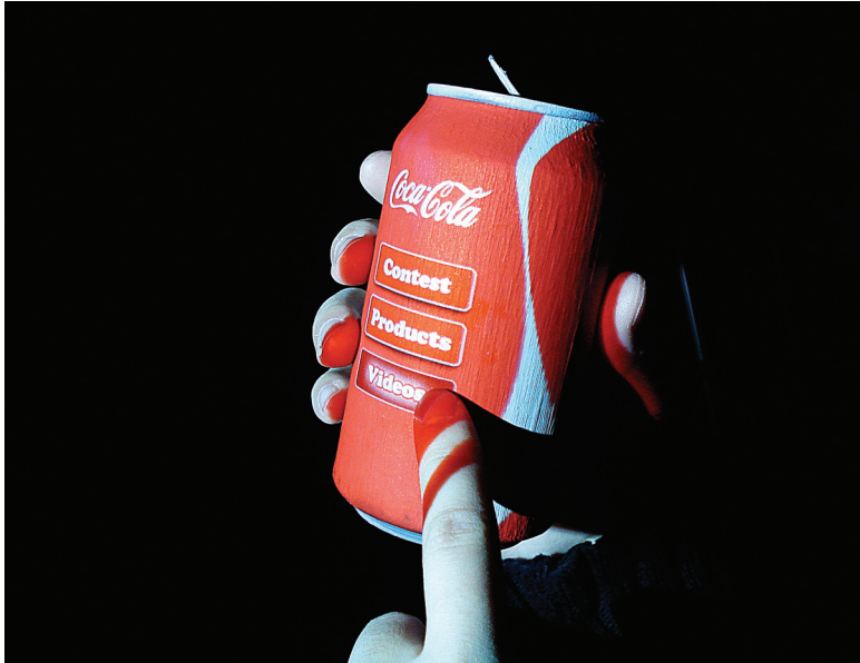
► Figure 2. Dynacan is an interactive curved computer on a pop can. To underscore the issues with recycling such computational objects, its skin was made out of projected reusable photons, rather than FOLEDs.
