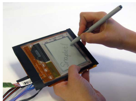
Figure 2. Snaplet held flat changes to a PDA with pen-based note taking functionality.
