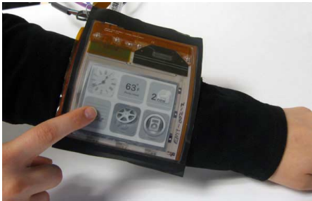
Figure 1. Snaplet, when worn in a convex shape as a wristband, switches its application context to watch and media player functionality.
