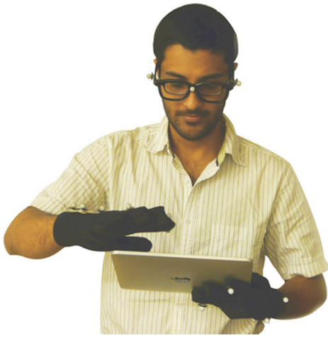
Figure 3. VJ, with glasses and gloves, throwing a video from the iPad onto the large display using a Swipe gesture.
