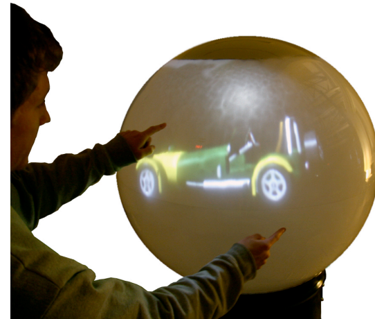
Figure 3. Scaling gesture. To scale a model, a user uses a two finger pinch. As the distance between the fingers increases, the models is enlarged as the distance decreases, the model is shrunk.
