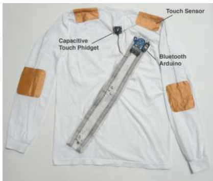
Figure 3. Interactive Lumalive shirt with touch sensors: front (top) and back (bottom).
