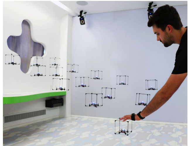
Figure 1. GridDrones system with an array of self-levitating physical voxels represented by small quadcopters.
