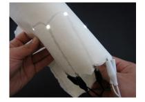
**figure 2.** Composite combining natural paper and electronic components [2].
