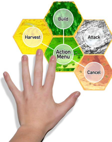
Figure 1: Hexagonal OLED displays simulated through tracking and projecting on cardboard tiles. Here, a marking menu is displayed on surrounding tiles upon obscuring an IR marker.
